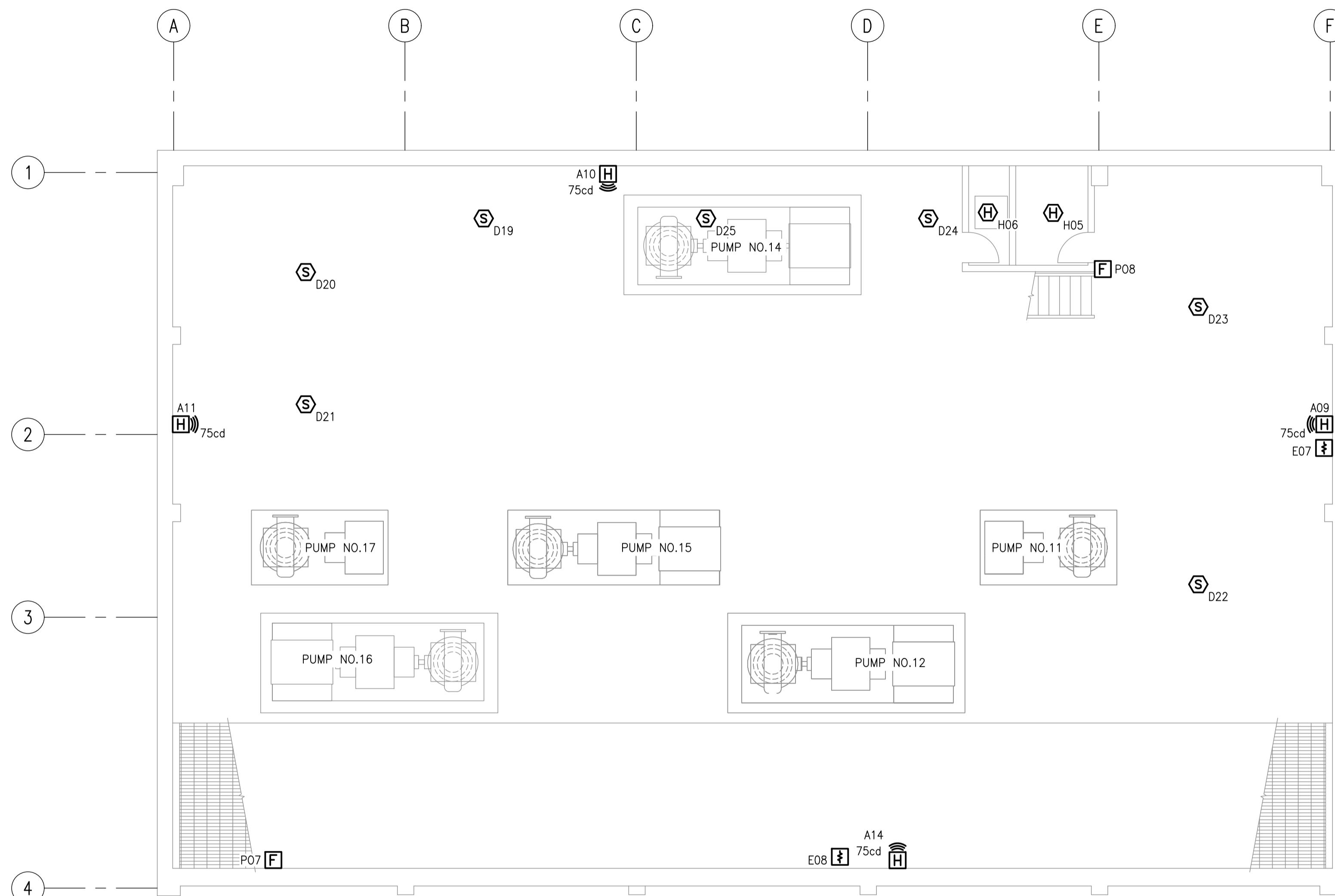
PUMP FLOOR FIRE ALARM PLAN - ELEV 229.220
